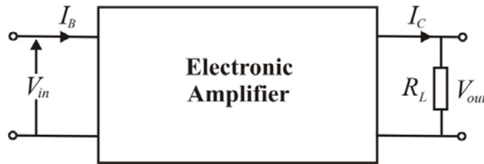
Figure 2. Simplified representation of an electronic amplifier with transistors or integrated circuits.
